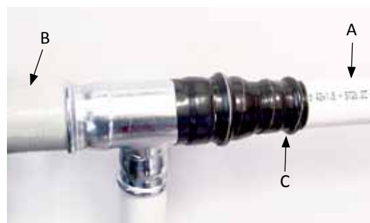
Figura 36 - Protection against external corrosive materials: A. Pipe with PP-coating B. Varnish with primer C. Protection with butanol adhesive tape
